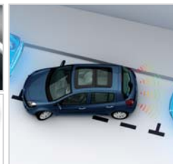
PARK DISTANCE CONTROL SENSORS Detects obstacles which could be impacted by the vehicle whilst reversing.
